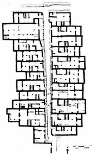
Street Layout in Jaisalmer, Rajasthan: The north-south-running street assures that only a narrow front of each house is exposed to the most critical summer sun that comes mainly from the east and west. Tall houses facing each other across the narrow street also provide a mutual shield. ( Paradigms of Indian Architecture by G. H. R. Tillotson 1998, 162.)
